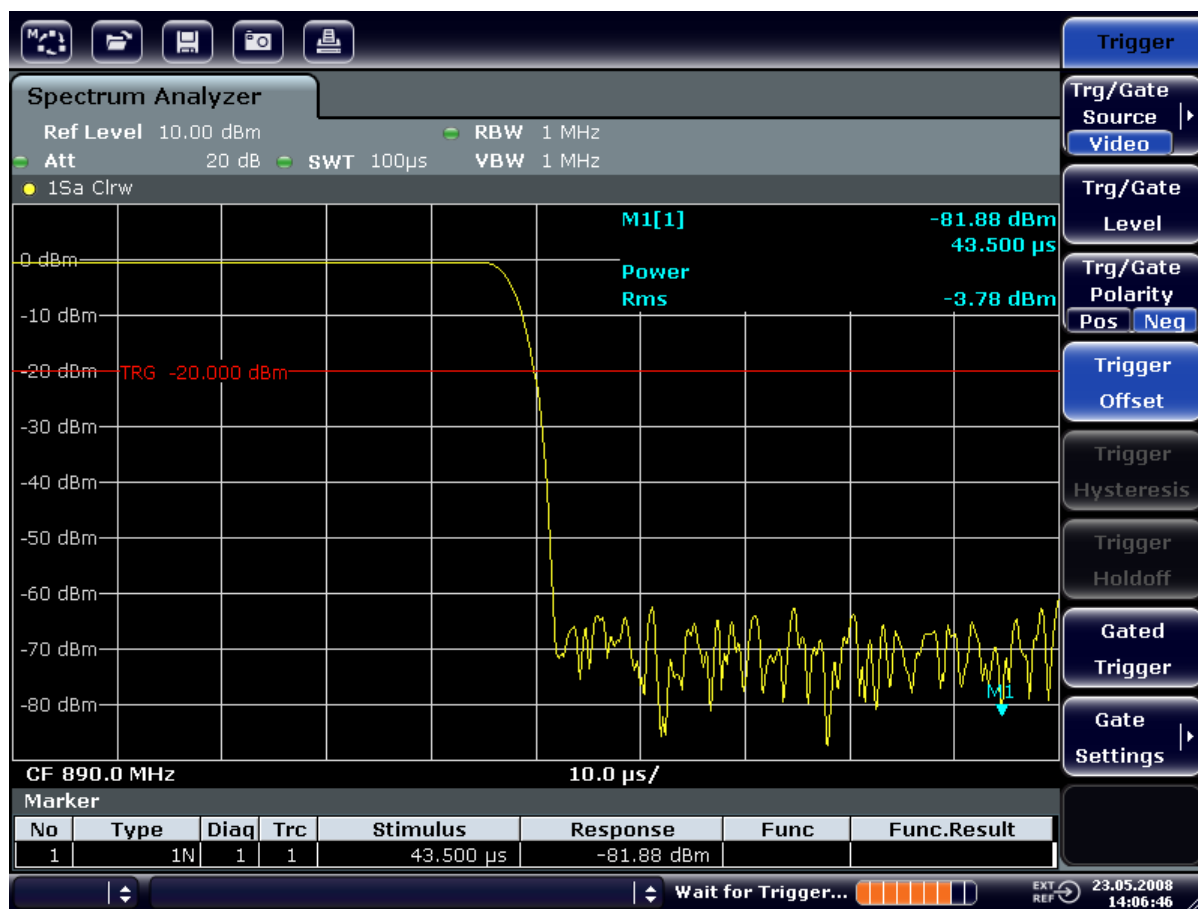
Fig. 6-18: Falling edge of the GSM burst displayed with high time resolution
